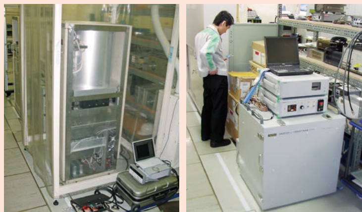
Atomic clock (left: haydrogen maser, right: caesium)
