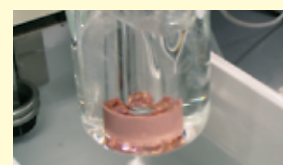
Figure 1 Removal of Cu(II) ion from aqueous solutions by the photoreduction on TiO 2 film.
