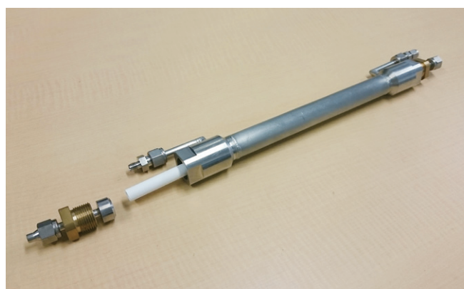
A tubular inorganic nanoporous membrane and a membrane module
